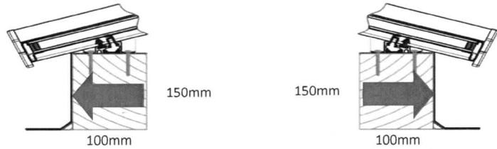
The required timber upstand size is **100mm x 150mm**
